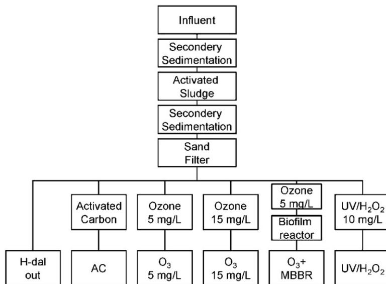
Figure 3. Scheme of the treatment technologies at Henriksdal STP. H-dal out feeds the different post-treatment processes.
